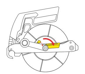
Push the lever forward to dis-engage drag. This also lets the pawl engage to stop reeling out.
